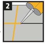
As soon as possible after application, smooth the grout with a finishing tool (metallic ball) to obtain a smooth finish
