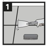
After making sure that the two components are blended well, extrude SikaCeram®-850 Design into the joint ensuring that it comes into full contact with the sides of the joint and avoiding any air entrapment
