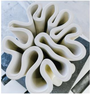
Sika's 3D concrete printing technology allows complex geometries to be realized economically.
