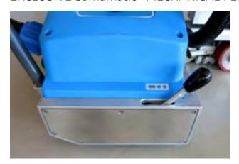
Neutral gear for easy moving on the roof.
