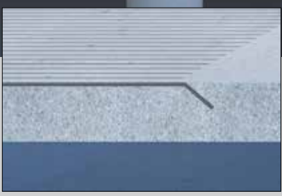
SikaWrap® FX for anchorage of near surface mounted (NSM) cantilevered applications
