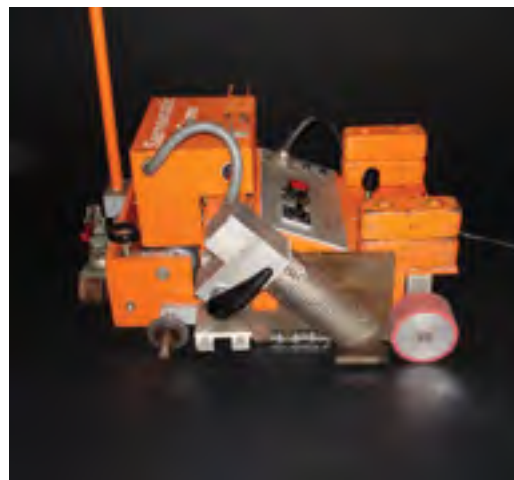
1966, Invention of Sarnamatic® Seam Welder: Sarnafil® was the first membrane manufacturer to design and produce an automatic seam welder, recognising early on that seam integrity was critical to the long-term performance of thermoplastic roofs.
